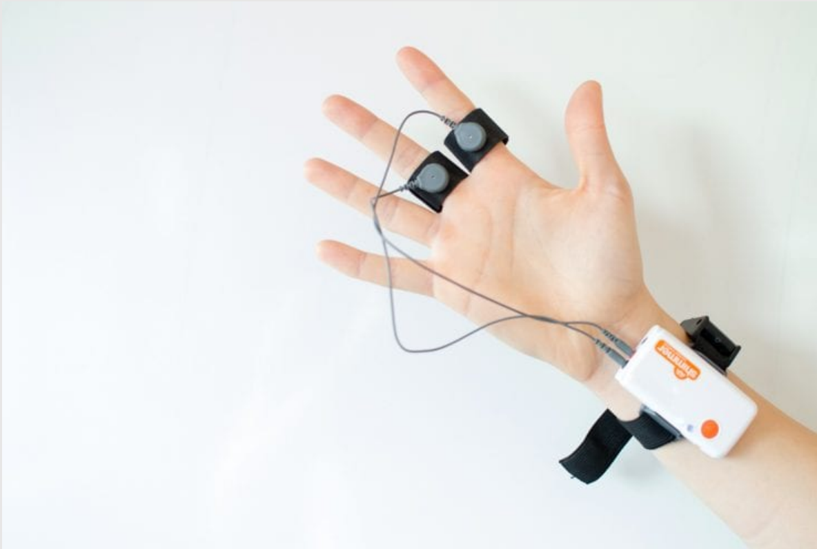
EDA sensor and electrodes
